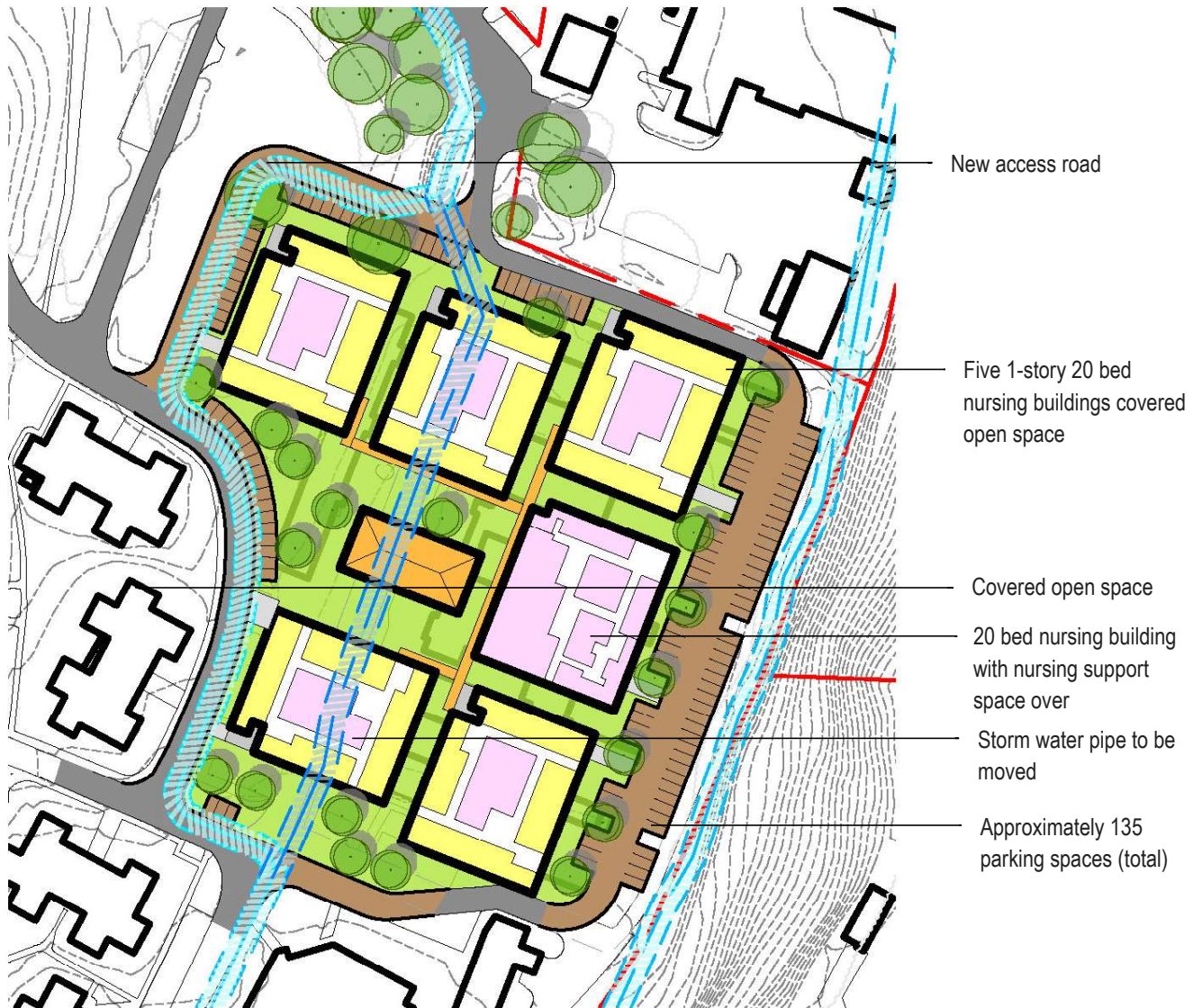
Area 1 NE 1-Story Nursing Facility Conceptual Site Plan(pipe move) Fircrest School Land Use Assessment
