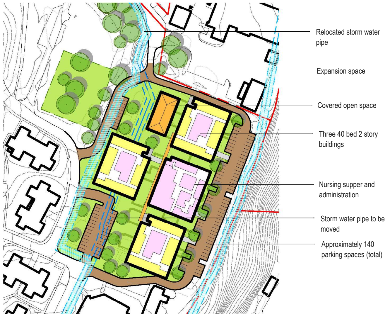
Area 1 NE Nursing Facility (2-story pipe move) Conceptual Site Plan Fircrest School Land Use Assessment
