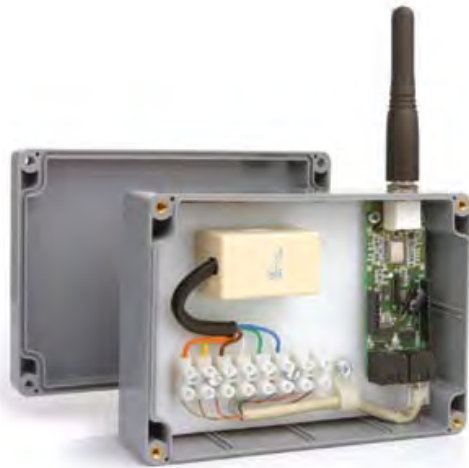
R-2000-S Serial Reader (Shown in a 2NEM Enclosure)
