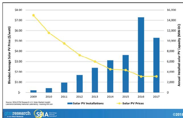
Figure 4: Solar PV Installation Cost & Installed Capacity (SEIA, 2018)
